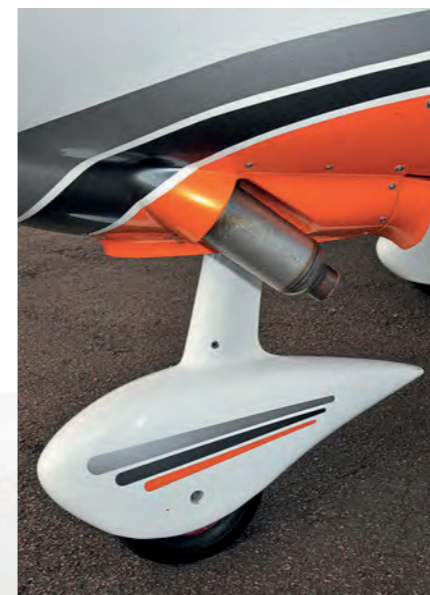
▲ The mainwheels are mounted on spring legs attached to the fuselage and are fitted with hydraulically operated Beringer disc brakes
