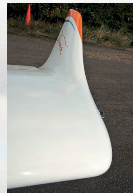
▲ Aerodynamic refinements for the seventh generation Dynamic include new, smaller winglets
