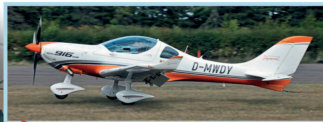
▲ Because of the crosswind, only 'Flap 2' was used for landing. The slightly higher approach speed of 60kt ensured the aircraft retained plenty of control authority right into the flare
