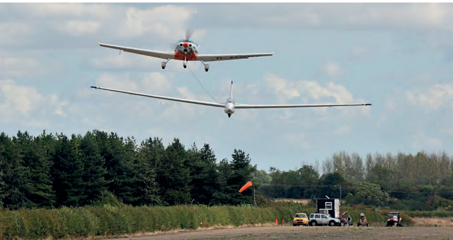
▲ The new 916iS-powered WT-9 tug made easy work of the two-seat SZD-54 Perkoz from Saltby's hard runway
