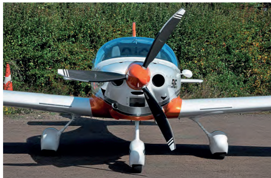
▲ The three-blade constant speed hydraulically actuated Woodcomp propeller features scimitar-shaped blades. The test aircraft had annular conspicuity lights around the circumference of the engine cooling intakes
