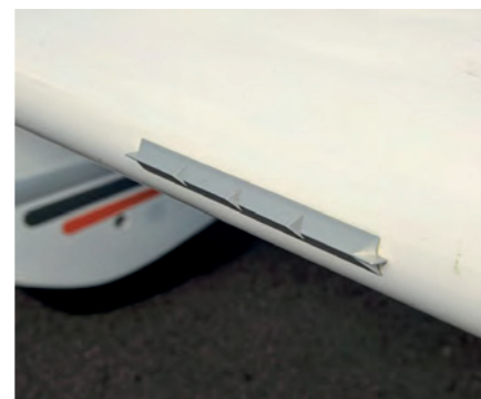
▲ One of the unusually sharp-edged 'Toberone' stall strips, mounted both mid-span and inboard, near the root
