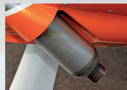
▲ The steerable nosewheel is carried by a steel tube attached to the firewall supports, suspension provided by bungees and a rubber bloc damper ▲ In the interest of reducing the noise footprint the new 916iS installation incorporates a massive exhaust muffler
