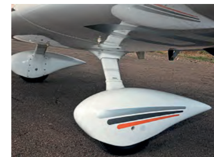
▲ The mainwheels are mounted on spring legs attached to the fuselage and are fitted with hydraulically operated Beringer disc brakes
